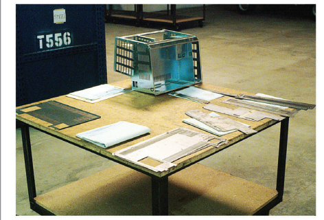
Finished Lisa sheet metal interior structural assembly with parts around it. Copyright © Bill Dresselhaus
