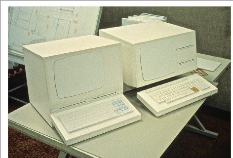
Two early somewhat boxy foam-core mockups of potential Lisa volumes/shapes. Copyright © Bill Dresselhaus
